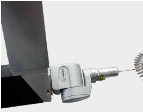
HP-O Flex 90 • Indexing head 2.5° mounted horizontally • For non contact blisk inspection
